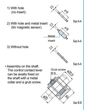
Assembly of Part. S0518 (with insert for magnetic sensor)
